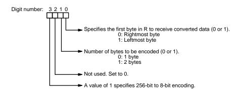
Three possible C values and the conversions that they produce are shown below. (In R, 0 indicates the rightmost byte and 1 indicates the leftmost byte.)
